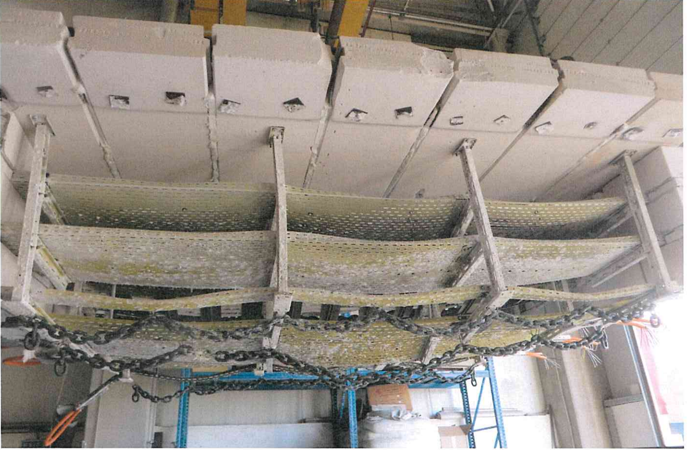
Photo B3: Exposed side of the test specimen after the test.
